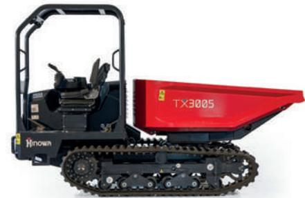
▲ Bucket larger and lower compared to the previous model granting a volume capacity of 1.49 m<sup>3</sup> (ISO 6483).
